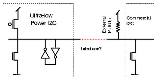
Figure 3: Two incompatible I2C implementations. Extreme care must be taken to not overpower the weak keeper. Driving signals to the low-power side requires manually driving the SDA line high both when writing and reading.
