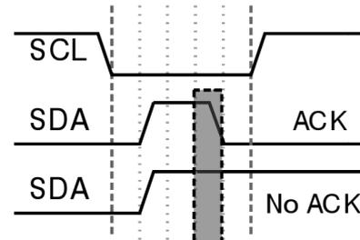
Figure 1: The ACK cycle of the modified I2C protocol. The negative clock edge is divided into 5 cycles: wait, pulse up, wait, pulse data, wait. These cycles are all 250ns long, permitting any clock rate up to 400kHz. The shaded region marks the only period in a I2C transaction the slave is responsible for driving.
