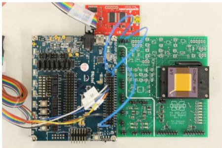
(a) The complete system: A commercial I2C device the BusPirate (top), the interface circuit realized in an IGLOO nano FPGA (left), and a breakout of the M3 control CPU board (right)
