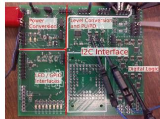
Figure 4: A combinational approach to interfacing the two divergent I2C systems. The M3 pull-up signal is supplied to a monostable multivibrator acting as a one-shot timer
